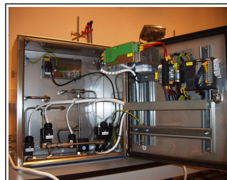
An inside view, with the mini PLC
